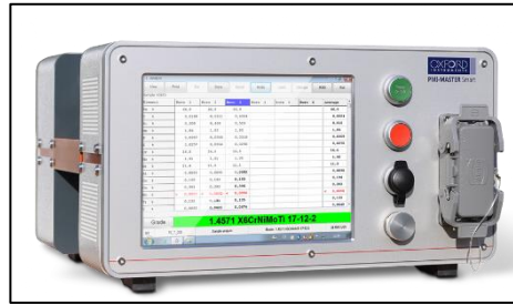
Fig. 9: Performing the optical Emission spectrometry Source: HWK-KO
