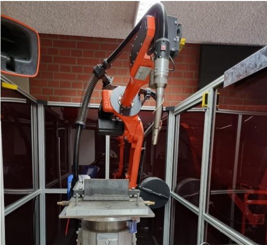
Fig. 10: Welding robot in articulated arm design; Photo HWK-Ko
